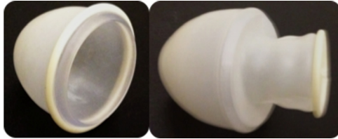
Fig. 2 Revised design. Left: shell with non-deployed latex rolled at the groove. Right: shell with deployed latex.
